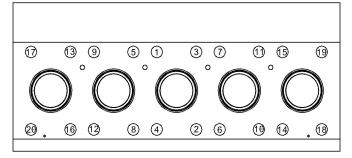
FIGURE 4-1 GD-2500Q Fluid End Tightening Sequence
