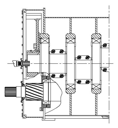
FIGURE 2-3: GD-2500Q Power End Rear Section View
