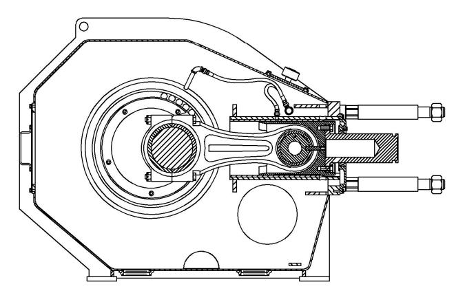
FIGURE 2-2 GD-2500Q Power End Section View
