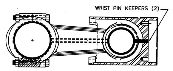
FIGURE 4-4 Crosshead Assembly
