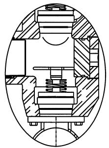
FIGURE 4-3: Fluid End Valve Stop
